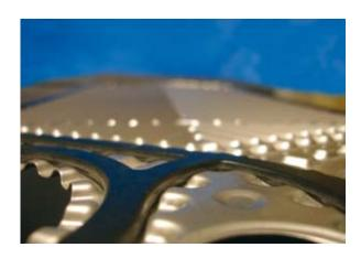
High performance plate type heat-exchangers consist of a number of formed, sealable heat-exchange plates according to the respective requirements. The alternating pressed plates and channel spacing cause highly turbulent flow behaviour, optimal self cleaning effect and highest possible heat transfer.
