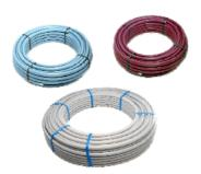
I-APEX is a multilayer pipe suitable for the distribution of hot and cold potable water, heating and air-conditioning systems. I-APEX pipe features a 5-layer structure in which a butt-welded aluminium pipes is contained between two layers in cross-linked polyethylene, being the layers bonded together by adhesive layers. Available in rolls, with or without blue or red insulation.
