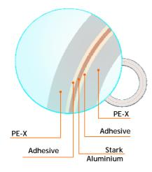
The two plastic layers in I-APEX pipes are made of crosslinked polyethylene PEX-b. This crosslinking method consists in creating chemical bonds by the addition of silanes during the extrusion process and by the immersion of the extruded pipes into a hot water bath (about 70-95  $^{\circ}$ C).
